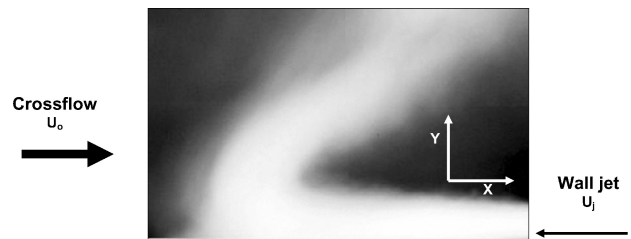
Fig. 2 Visualization of the flow, U_j = 6 m/s and U_0 = 3.48 m/s.
